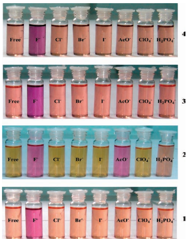
Figure 7. Color changes that occur when the solutions of 1–4 are treated with various anions as their tetrabutylammonium (TBA) salts.
